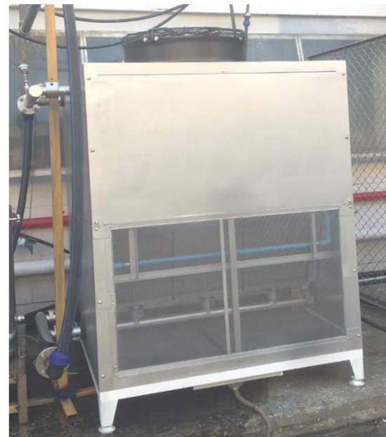
Closed circuit cooling tower (Water spray with high heat transfer cell)
